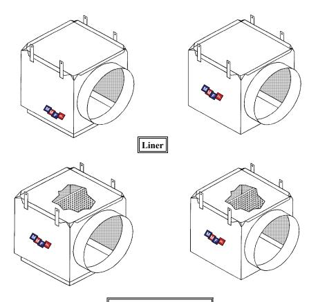
Liner - Perforated Baffle
