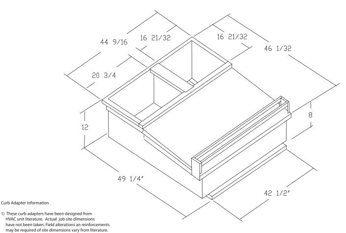
2) Before ordering curb adapter, contractor must confirm that dimensions of existing curb on job site matches dimensions of existing curb on this drawing.
